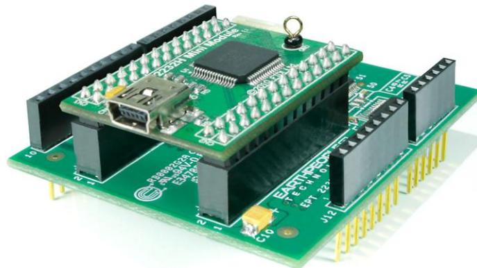
An on board 66 MHz oscillator is used by the EPT Active Transfer Library to provide data transfer rates of 8 Mega Bytes per second. Twenty Four I/O's from the CPLD are attached to three 8 bit transceivers to provide 5 Volt compatible I/O's. These 74LVC245 bidirectional voltage translator/bus transceivers are controlled by one enable and
