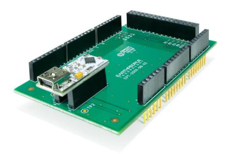
The EPT 220X-DB-M4 is designed to support the MEGA board of the Arduino Open source Prototyping Platform. The MEGA can communicate as an SPI Master to an SPI Slave device. The EPT 220X-DB- M4 is a USB to Slave SPI device. This will allows users to communicate from the Arduino MEGA board to the PC over SPI. Use the Active Host API to quickly and easily create a simulated SPI sensor on the PC. Use the simulated SPI Sensor to debug your Arduino SPI Master communication code.
