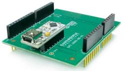
module. Both the Uno and the Serial Graph Tool can be powered up at the same time. The EPT 220X-DB-U2 board receives its power from the USB cable. To use the board, connect a USB
