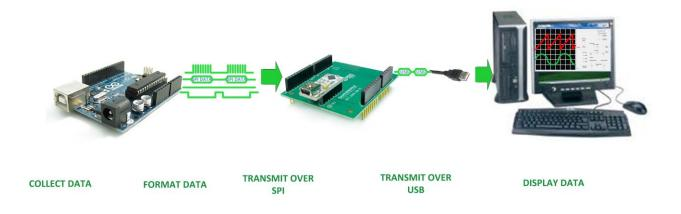
The EPT Serial Graph Tool makes it easy to graph fast or slow data coming from the Arduino Uno. The user only has to write code for the Uno. Just collect the data into an array then send the array and channel number to the EPT 220X-DB-U2, then send the end of frame command. There are only two functions needed to display data on the Serial Graph Tool.
